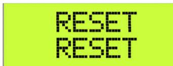
When Mach3 is in Emergency mode and the E-STOP button is in reset position, “RESET” on LCD flashes at ½ second rate.
